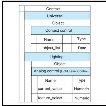
Figure 1—Here's the CEBus context specification for the receive-only relay. Most of a normal context specification is not necessary.
