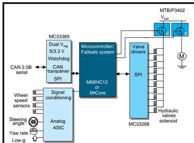
**Figure 5**—If a master and a slave microcontroller are implemented and the slave only performs plausibility checks, the configuration is asymmetrically redundant.
