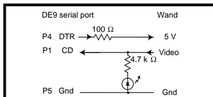
**Figure 2**—Because the PC serial port is rated to source 10 mA per pin, I can tap more than enough power off DTR. As a bonus, this unorthodox interface leaves the Rx/Tx lines free for other applications.
