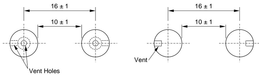
**Figures 3 and 4 – Alternative forms of vented electrodes**
