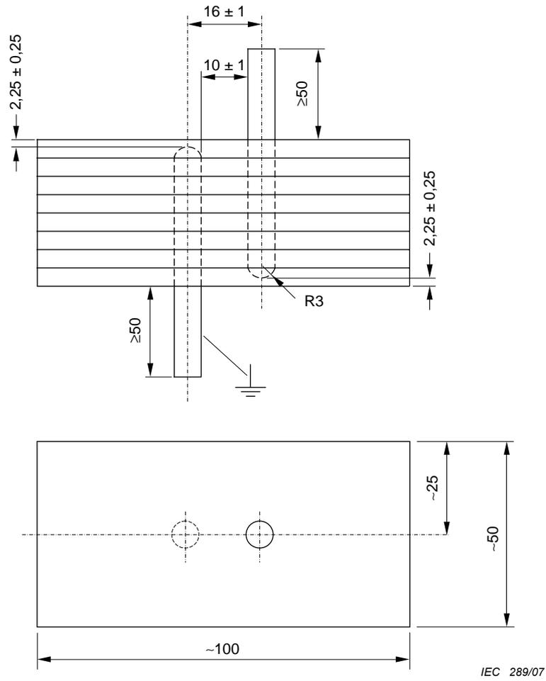
**Figure 2 – Size of the test specimens and arrangement of the electrodes for testing the electric strength along laminae (edgewise electric strength)**
