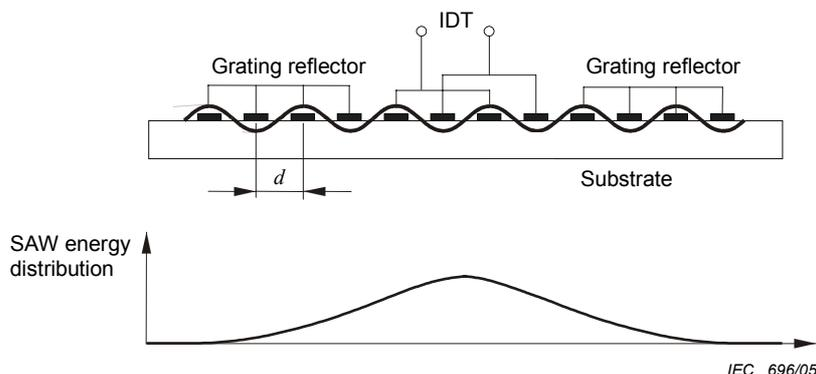
Figure 3 – Standing wave pattern and SAW energy distribution
