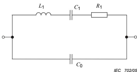
$$f_s = \frac{1}{2\pi\sqrt{L_1 \times C_1}} \quad \text{is the motional (series) resonance frequency;}$$
