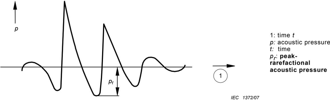
**Figure C.4 – Schematic diagram illustrating the peak-rarefactional acoustic pressure during an acoustic pulse**
