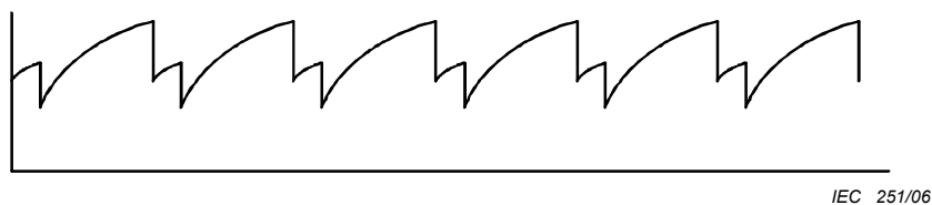
Figure 6c – Load communication: line-to-earth voltage
