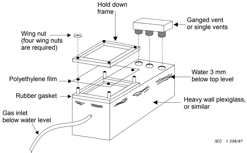
Figure 1 – Test fixture
