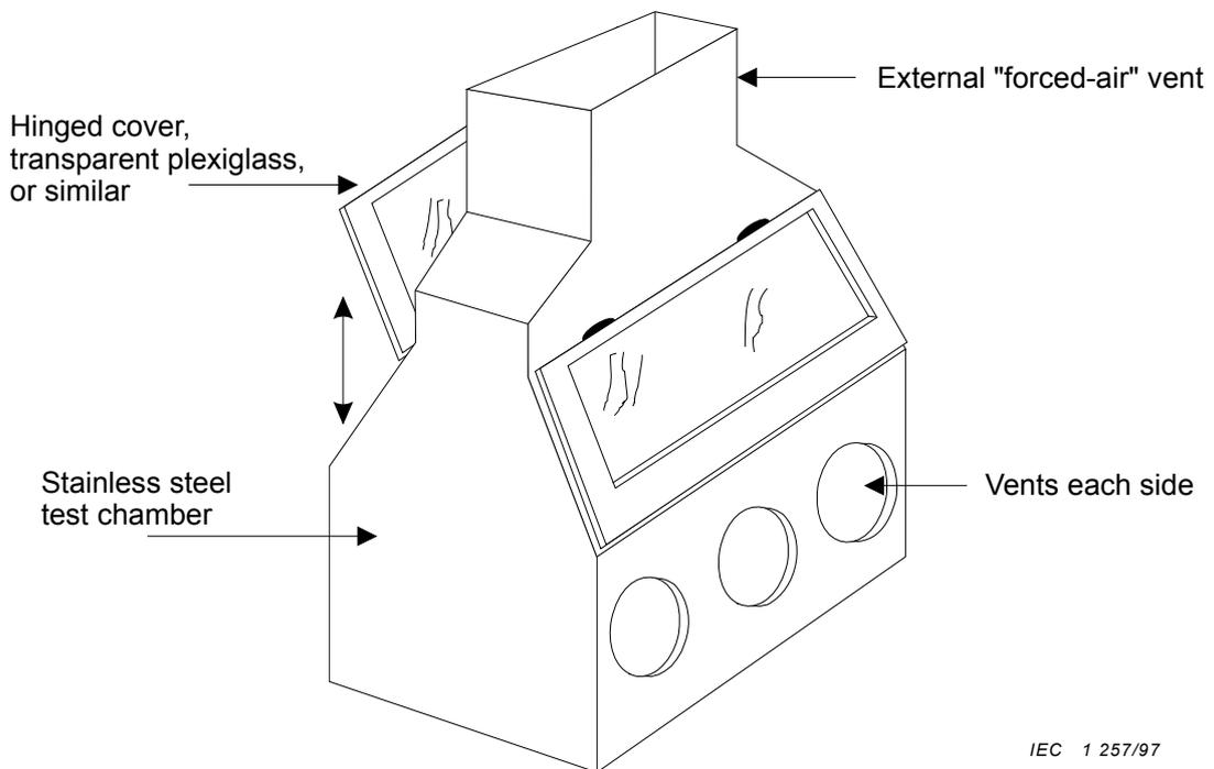
NOTE – This illustrates the essential facilities only. The plan area of the chamber should be approximately twice that of the test battery.
