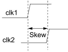
Figure 21 – Skew timing check
