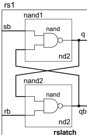
Figure 14—RS latch in a pin-to-pin modeling style
