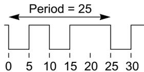
**Figure 31—Specification of a waveform of period 25**
