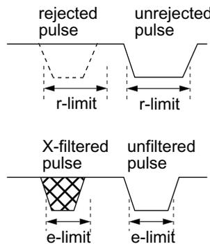
Figure 4—Pulse limits (r-limit and e-limit)
