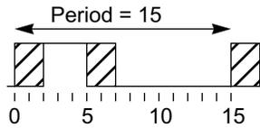
**Figure 30—Specification of a waveform of period 15**
