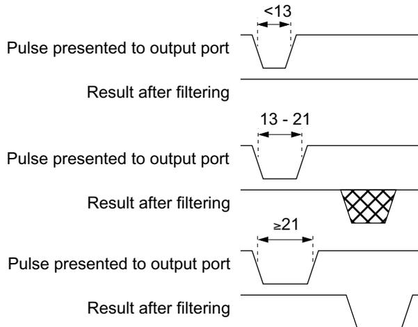
Figure 5—Pulse filtering
