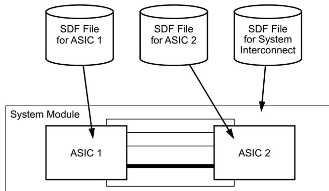
Figure 1—Multiple SDF files in a hierarchical design
