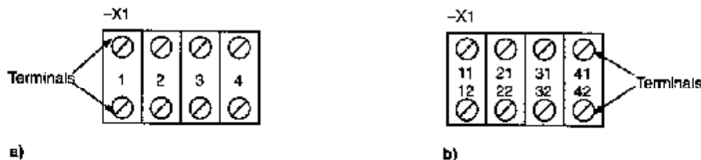
Figure B.2 - One terminal block with eight terminals (the complete unit is an object)
