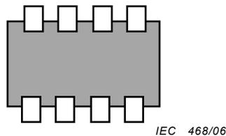
**Figure 6 – Terminals arranged peripherally in two rows**
