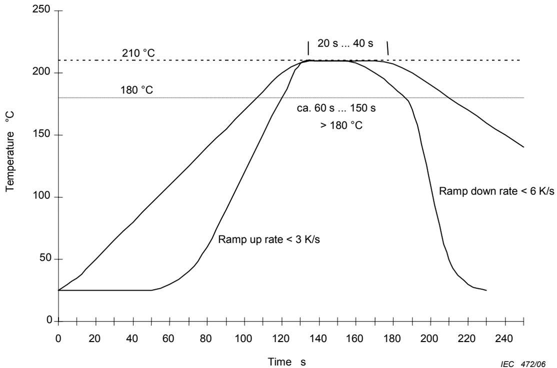
NOTE The lines indicate upper and lower limits of typical processes.
