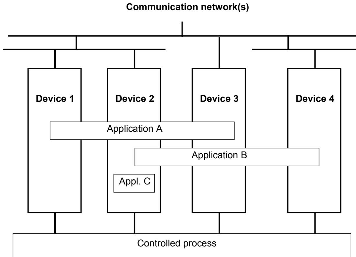
**Figure 3 – FB structure may be distributed between devices**
