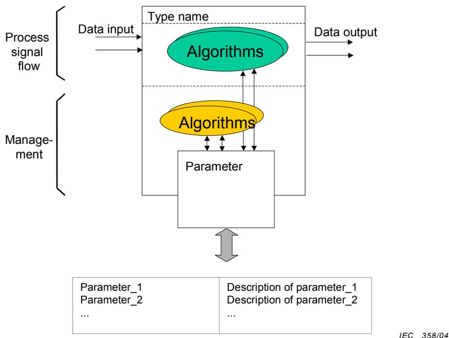
**Figure 7 – IEC 61804 block overview (graphical representation not normative)**
