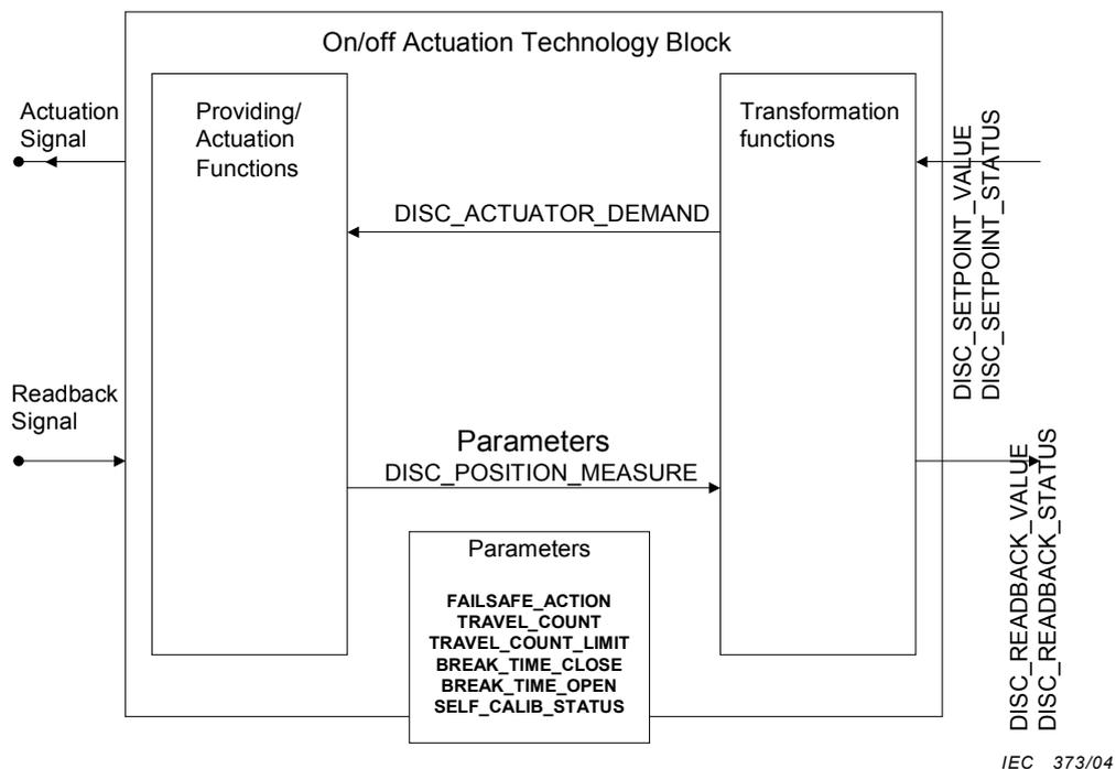
Figure 21 – On/Off Actuation Technology Block
