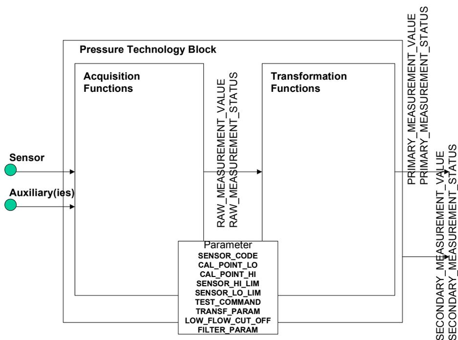
Figure 19 – Pressure Technology Block
