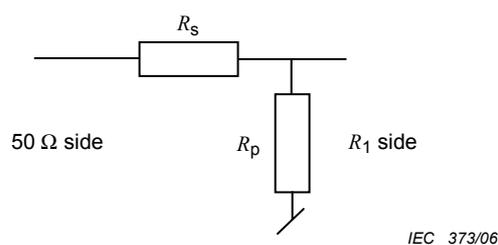
**Figure 7 – Impedance matching for  $Z_1 < 50 \Omega$**
