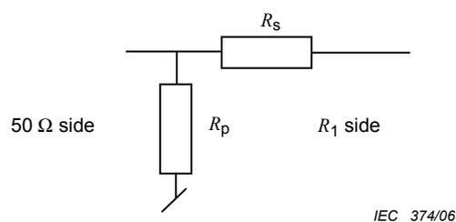
**Figure 8 – Impedance matching for  $Z_1 > 50 \Omega$**
