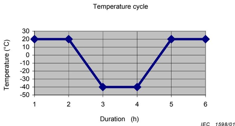
**Figure 3 – Temperature cycle inside chamber**
