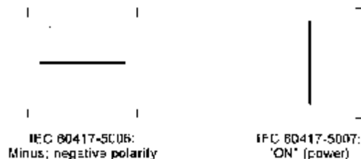
Figure 8 – Example of a graphical symbol the meaning of which depends upon its orientation
